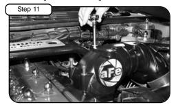
With 6mm hexagonal bit provided and 6mm socket, install the four mounting screws. Do not tighten completely!
