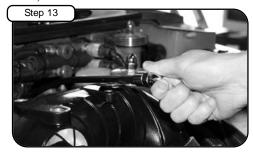
Install the engine oil dipstick using M8 socket cap screw provided. Tighten using 6mm allen key (See notes 1, 2 & 3). Attach the engine wire harness to the aFe manifold.
