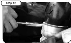
Tighten coupler hose clamp with 11mm socket (See notes 2 & 4). Tighten the four mounting screws from Step 11 (See notes 2 & 5).
