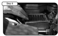
Remove both top and bottom stock gaskets away from air grid heater. Replace with new gaskets provided. (May require a scraper or scotch brite to clean sealing surfaces.)
