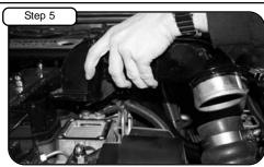
Carefully remove stock manifold out of vehicle. ( *Place a clean shop rag over air grid heater to prevent anything from entering* )
