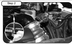
With a 11mm socket with ratchet, loosen the intercooler coupler hose clamp. Remove the engine oil dipstick screw with 10mm socket.
