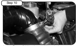
Insert aFe manifold into intercooler coupler hose.
