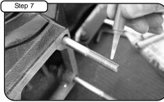
Install 1/8" NPT plugs to aFe manifold using 3/16" allen key. Apply threadlocker to the four mounting screws.
