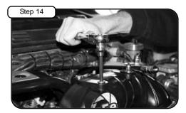
Install the two 3/8" NPT plugs to top of aFe manifold. Tighten using 8mm allen key (See notes 1, 2 & 5).
